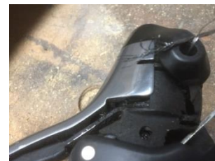
Frayed inner rear cluster cable, 3 strands from breaking
