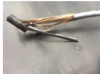
Split outer cable sheath, front ring shifter.
